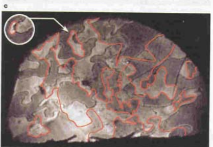
Figure 5 | Coexisting AFM and FTO domains of a \text{LiCoPO}_4(100) sample at 10 K imaged with SHG light at 2.197 eV. a, Obtained using light from Z_{\text{AFM}} . Dark lines are the AFM domain walls. b, Distribution of the AFM domains in a. c, Obtained using interfering light from Z_{\text{AFM}} and Z_{\text{FTO}} . Bright and dark areas are caused by the interference of AFM and FTO contributions to SHG (see text). Red lines indicate the FTO domain walls. Inset, FTO domain movement caused by a temperature cycle below T_N .
